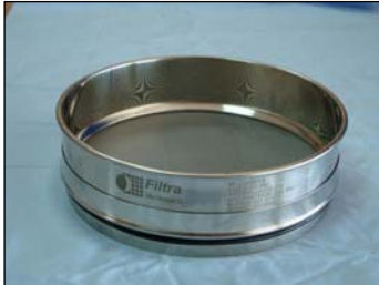
Sieves with stainless steel metallic mesh.
